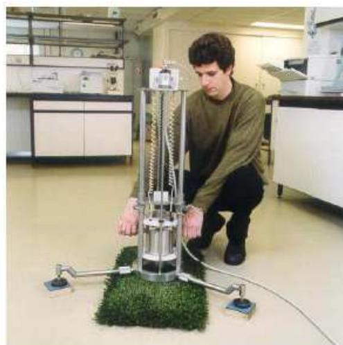
causes discomfort. We measure the stability of a surface by the amount of give in the surface, or **Deformation**. A weight is dropped onto a spring sitting on an anvil, as per the Berlin Athlete, but the weight and spring are different. Instead of measuring the force we measure the amount the
